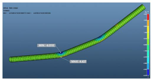
Figure 3. Pipe wall thickness on the inside expressed in mm, as determined by incremental solver simulation
