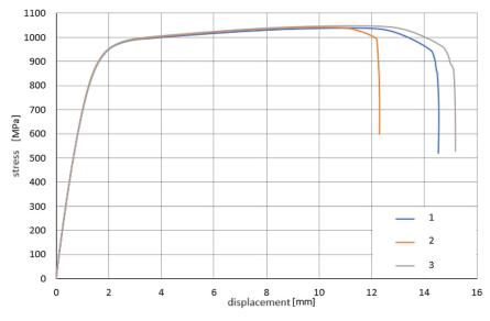
Figure 1. Uniaxial tension diagram of a sample made of steel 1.7734.5
