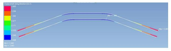
Figure 8. Springback as determined by incremental solver simulation
