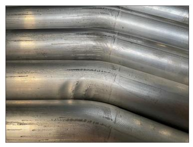
Figure 10. Forming defects in the form of folds of the inner radius
