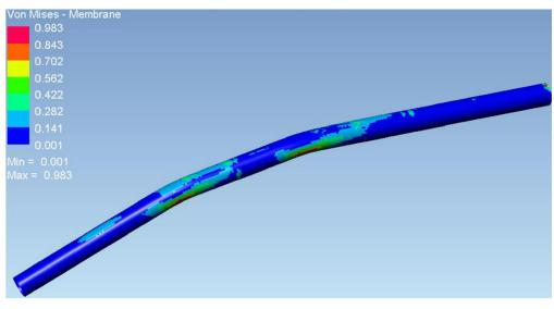
Figure 5. Stresses calculated according to the HMH hypothesis as determined by incremental solver simulation [GPa]
