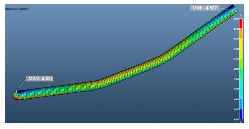
Figure 9. Springback as determined by one step solver simulation
