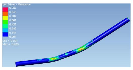
Figure 6. Stresses calculated according to the HMH Hypothesis as determined by incremental solver simulation [GPa]
