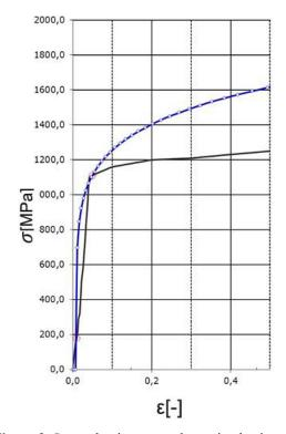
Figure 2. Strengthening curve determined using the Krupkowsky-Gesetz method for steel 1.7734.5
