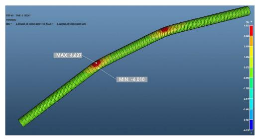
Figure 4. Pipe wall thickness expressed in mm from the outside, as determined by incremental solver simulation
