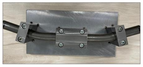
Figure 11. Verification of the geometry of the bent pipe in the device
